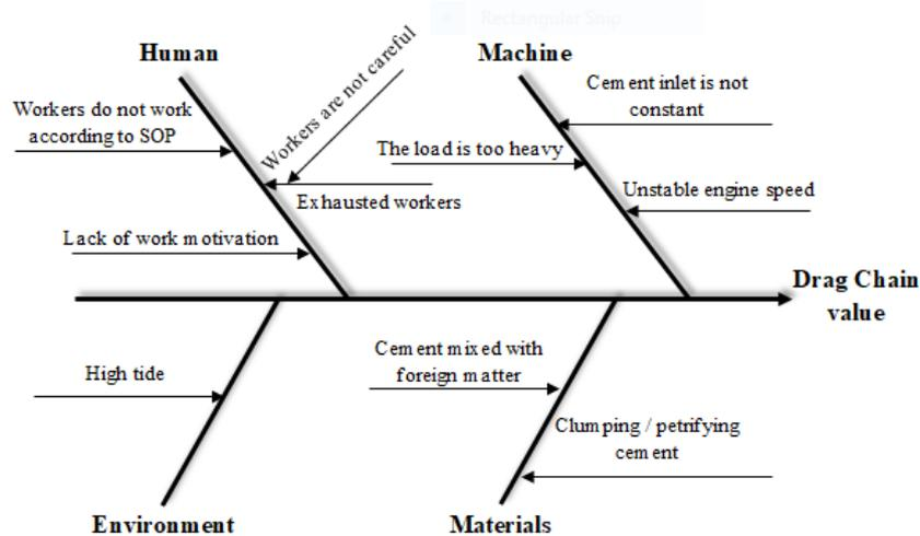
**Figure 6.** Fishbone Diagram drag chain performance
