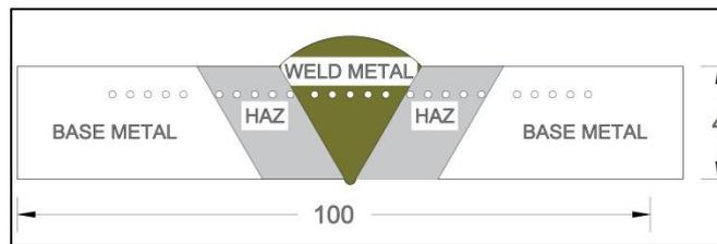
**Figure 3.** Micro-Hardness Test Coupon of AA1135
