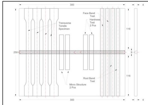
**Figure 2.** Schematic Of The Tensile Test, Bend Test, Hardness, And Microstructure
