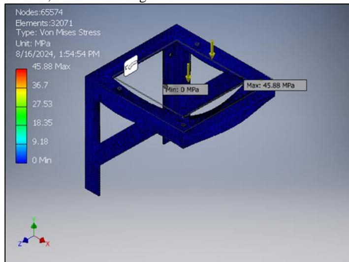
Figure 3.3 Von Mises Stress Simulation Result
