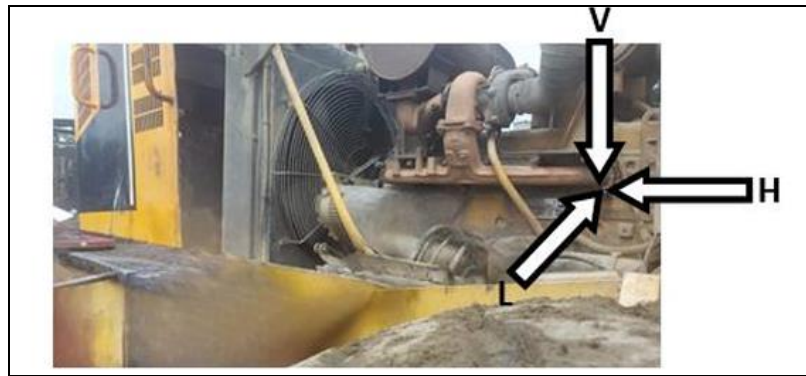
Figure 3.1. Noise Measurement Test in the combustion chamber of Wheel Loader engines with a distance of 100 cm, 150 cm and 200 cm with a capacity of coral stones of 3, 4 and 5 tons.
