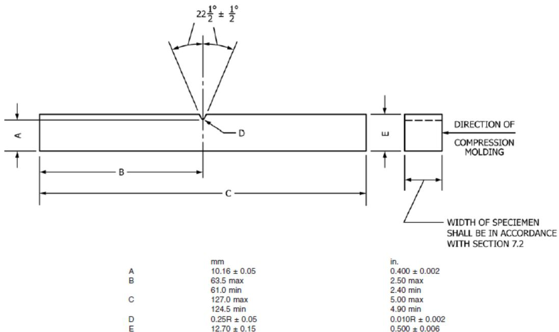
Figure 2.1. ASTM D6110-10 Charpy Impact Test Specimen Size [11][12].
