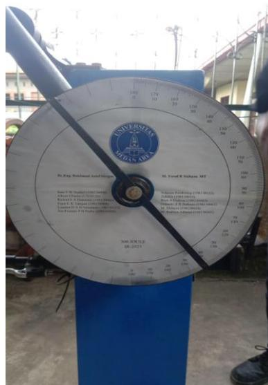
Figure 2.3. Position of the pendulum arm is 147 degrees.
