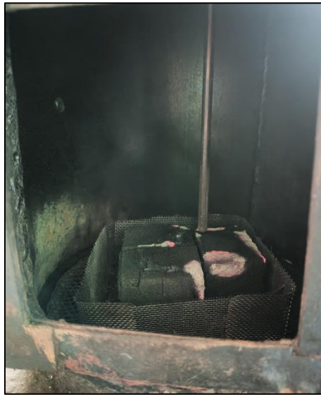
Figure 7 Briquettes after ignition using gas torch
