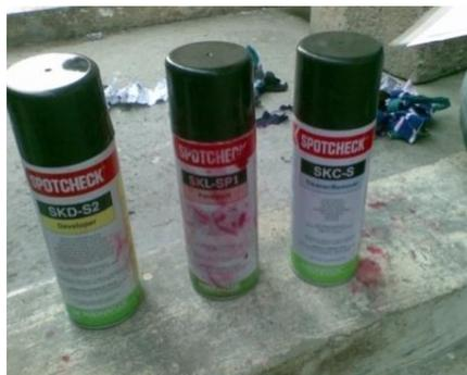
Gambar 3. Cairan Penetrant Test
