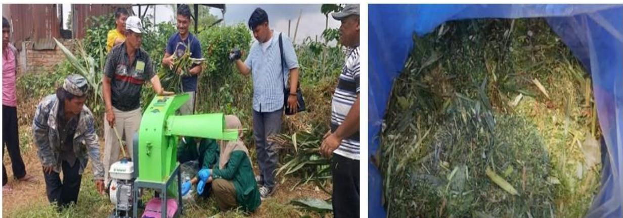
Figure 3. Maise straw chopping process using chopper machine for fermented feed making.
